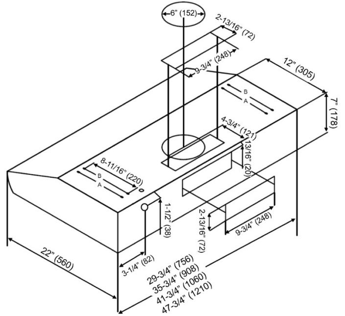
30 po = Trous de montage perçage " A "
