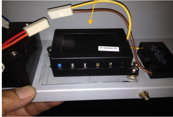
Figure 12: LED Driver Mounted
