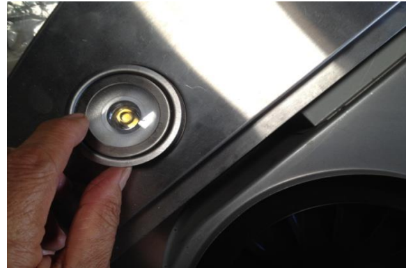
Figure 17: Push in LED Light into Position
