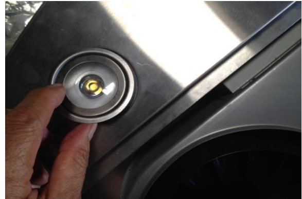
Figure 16: Push in LED Light Into Position
