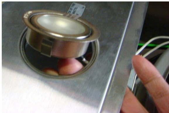
Figure 14a: Push the Halogen Lamp Inside Out
