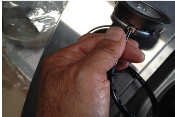
Figure 15: Connect the wire into the LED Light Socket
