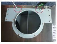
Step 4. Using the same 2 srews that were removed,install the Black Hood Mounting Bracket.
