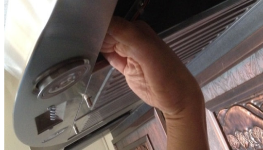
P2. Reaching from inside the hood push down on light fixture to dislodge it from its housing. Go to step 6.
